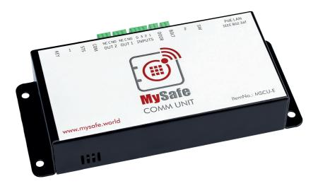
Depending on the settings, the device can block the opening of the safe and switch its outputs based on selectable lock events. The COMM UNIT is installed inside the security container and communicates with the outside world via Ethernet using an encrypted MQTTS connection. A single cable is sufficient for connection, as the device is powered via an Ethernet cable according to the PoE standard.
